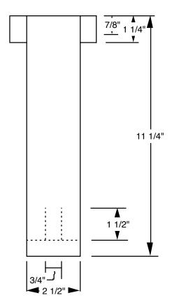
The frame support on the bottom is optional and is made from a piece of sheet metal.
