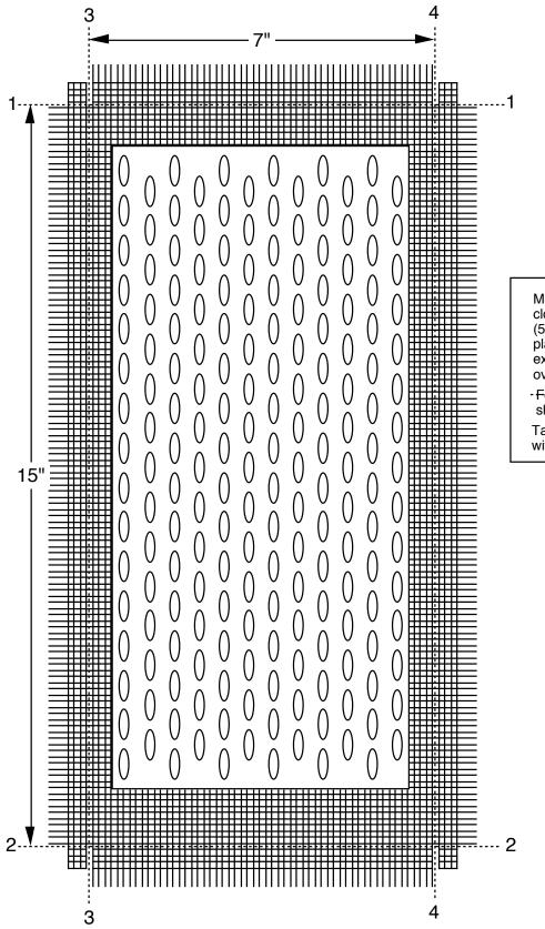
Material is 8 x 8 hardware cloth with the center cut out (5" x 12") and a piece of plastic or zinc queen excluder (6" x 13") fastened over it.
